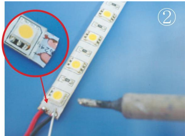
Remove silicone from the soldering pads and Solder the cable correctly. Please take care about correct polarity.
